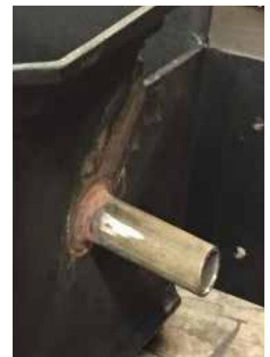
Example of hopper head fitted with spout (above) and in fabrication (right)
