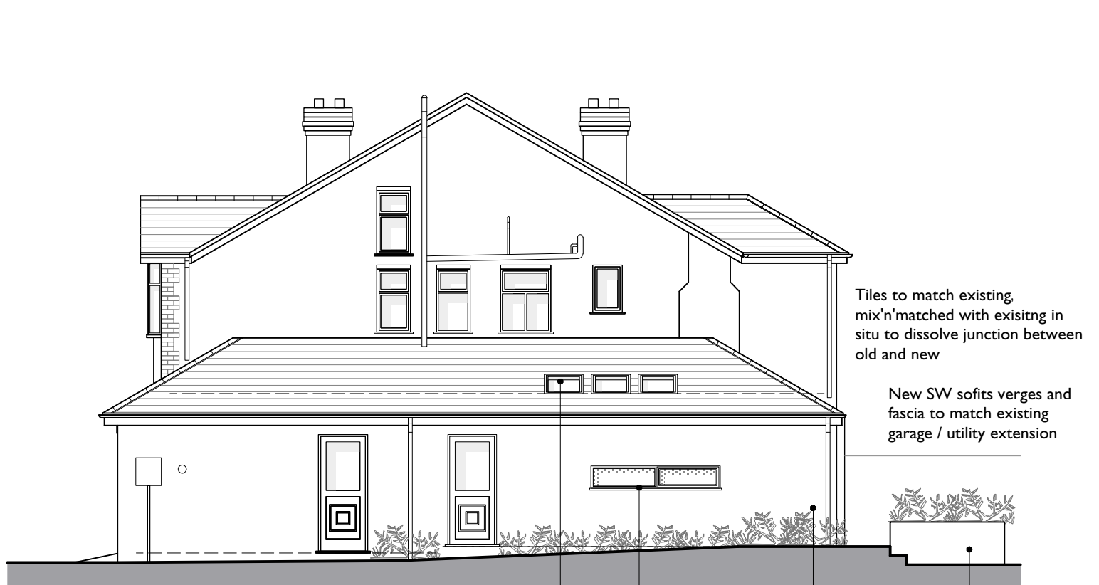
South West Elevation
