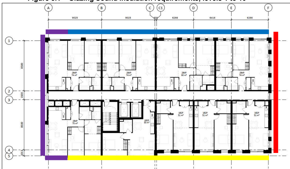
Figure 5.1 – Glazing Sound Insulation requirements, levels 1 to 10
