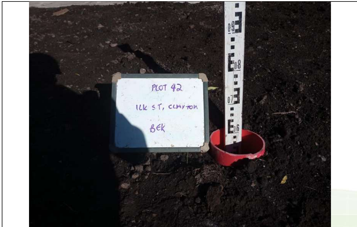
Photograph 1: Validation of Garden Capping Thickness
