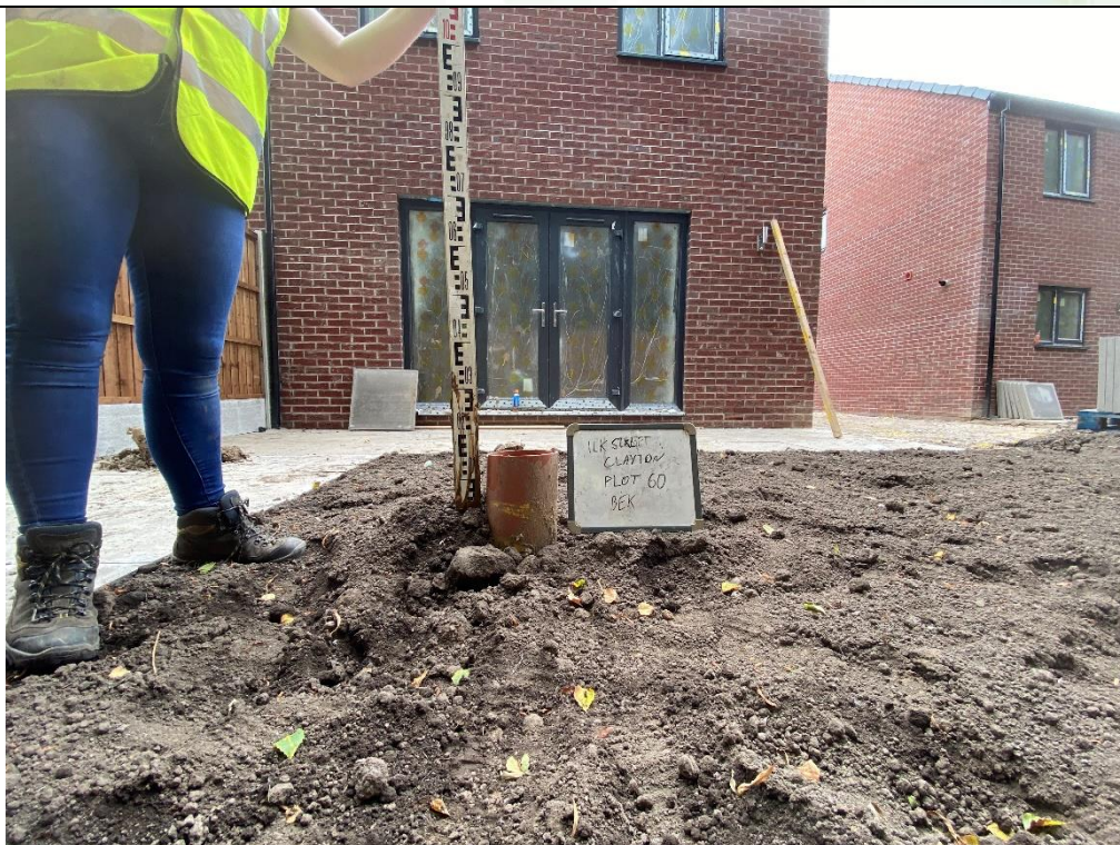
Photograph 2: Validation of Garden Capping Thickness (Plot 61, not 60)
