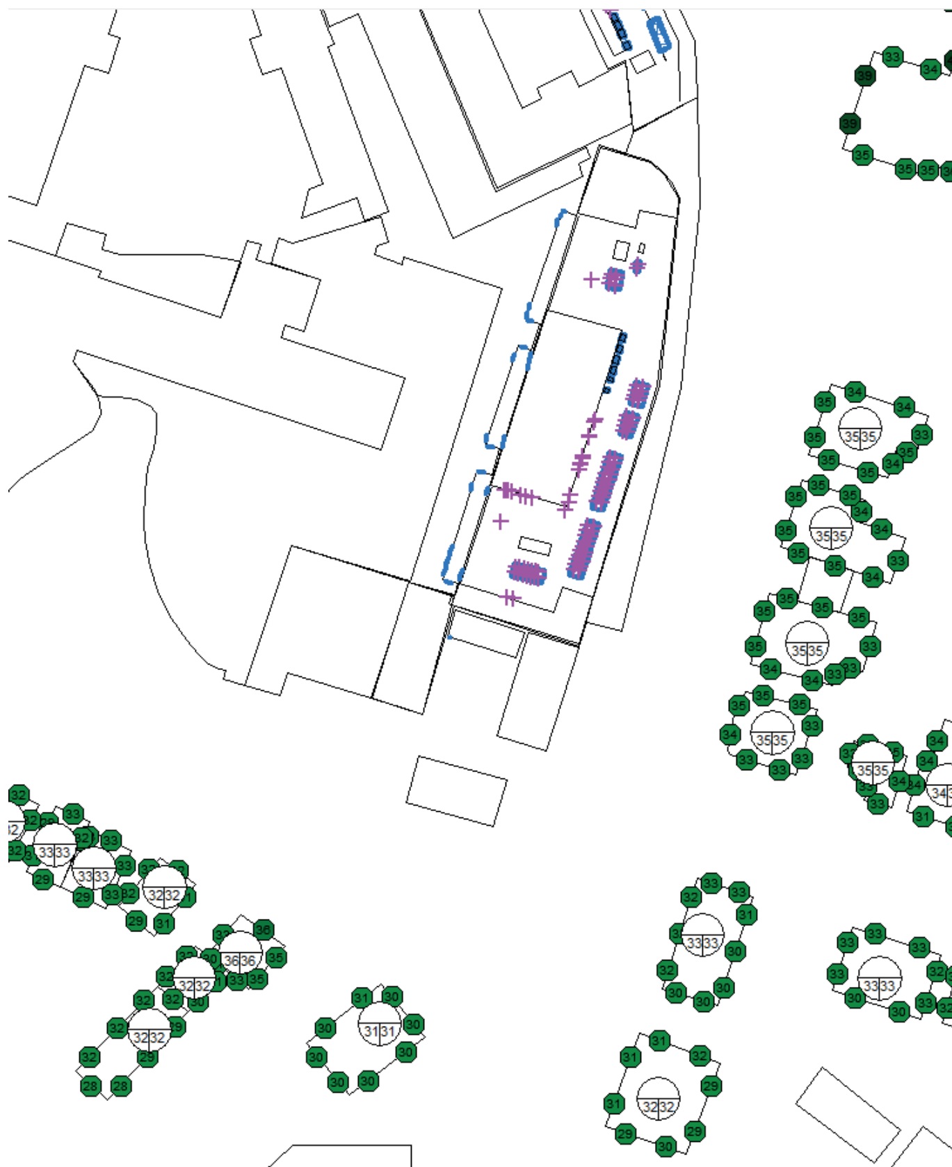
Figure 3: CadnaA model screen shot indicating the predicted plant noise levels ( L_{A,Tr} dB) at the facades of the nearest noise sensitive receptors
