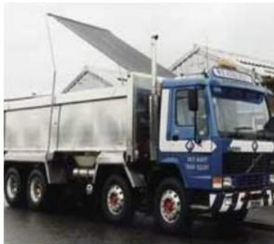
unrolling sheeting from front to back of the vehicle body (Fig.1)
