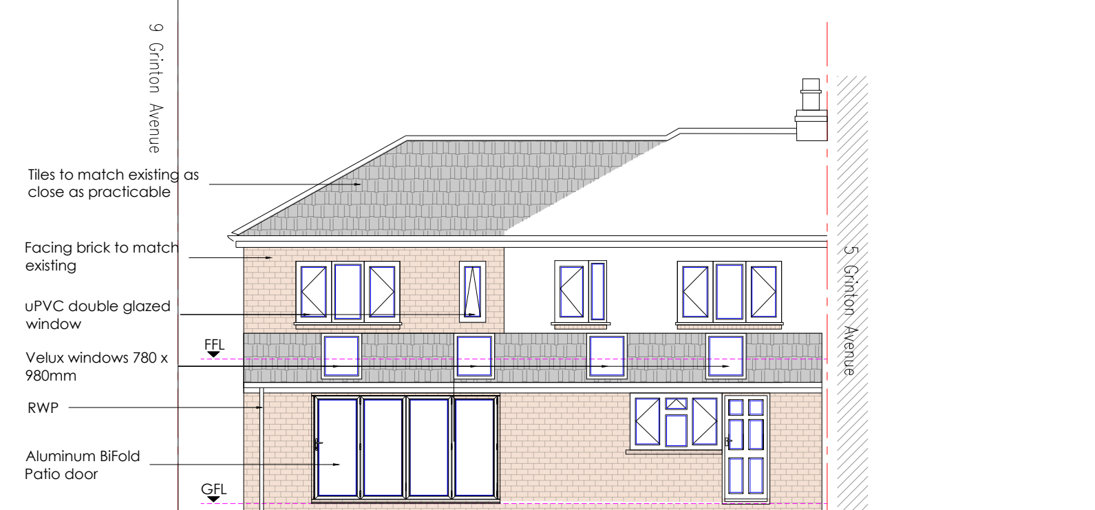
Proposed Rear Elevation Scale 1:100
