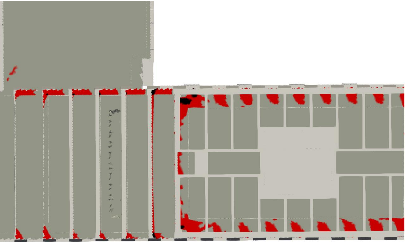
Figure Error! No text of specified style in document..22 Strong Winds at L26 Terrace and Southern Balconies for Proposed Development with Cumulative Surrounds
