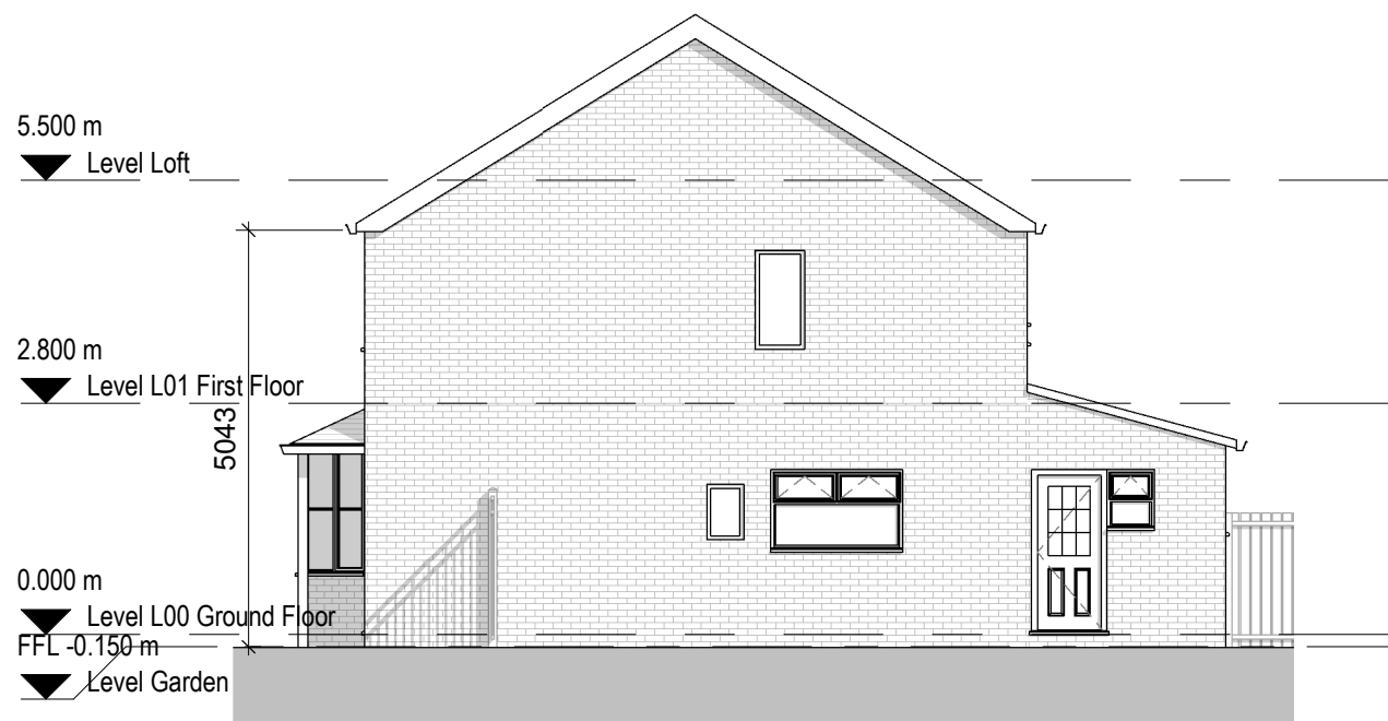
1 Existing West Elevation 1 : 100
