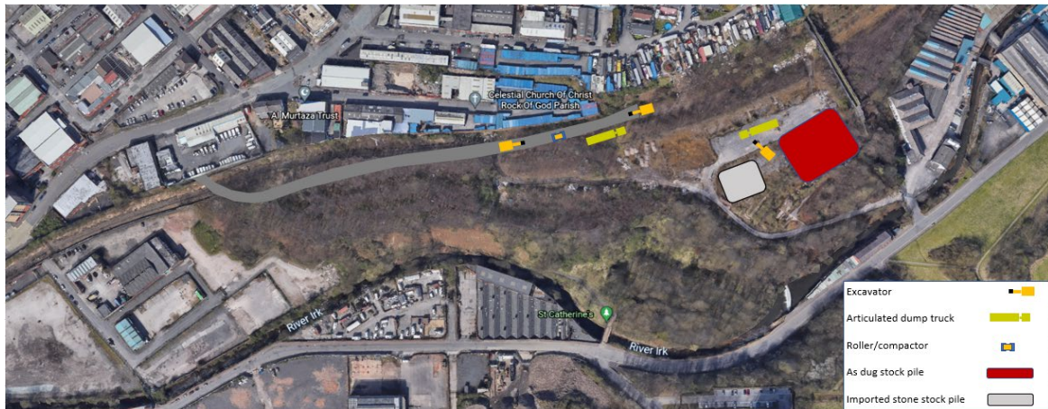
Stage 3 Works continue exchanging imported material for excavated
