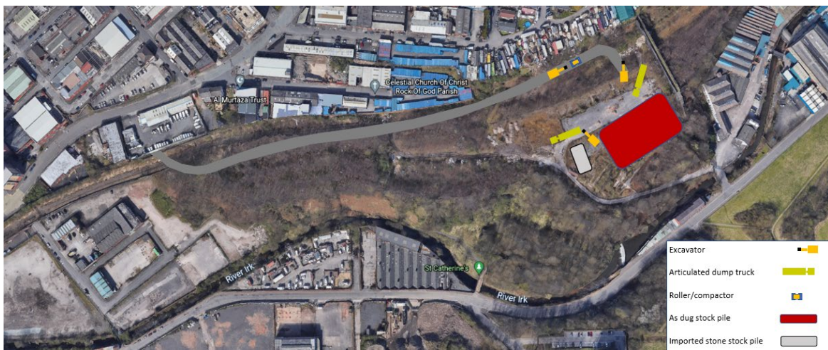
Stage 3 Works continue exchanging imported material for excavated
