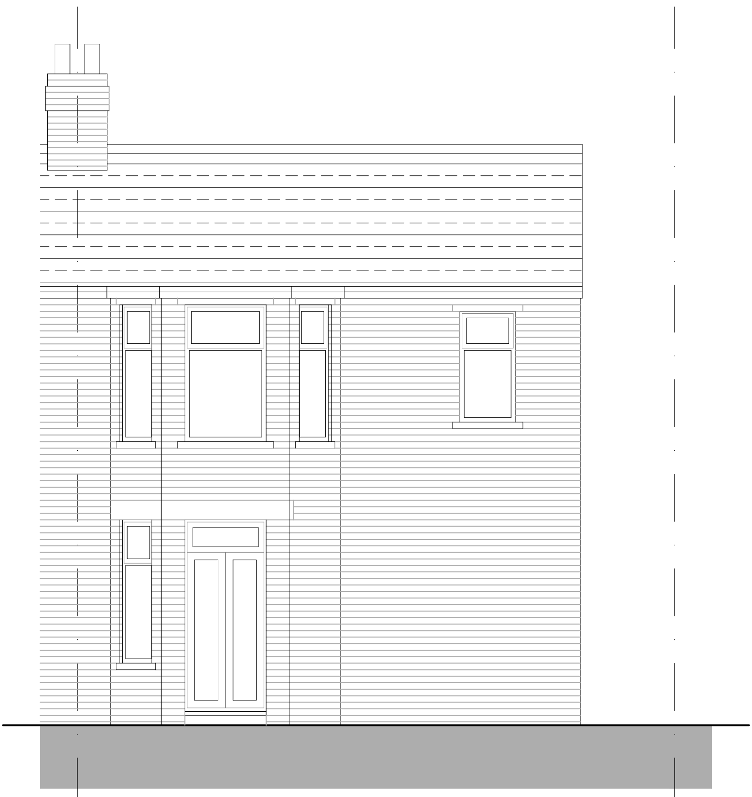
Existing Rear Elevation @ 1:50
