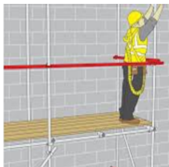
Pictures from NASC SG4:15 showing 'Scaffolders safe zone' and Scaff step.
