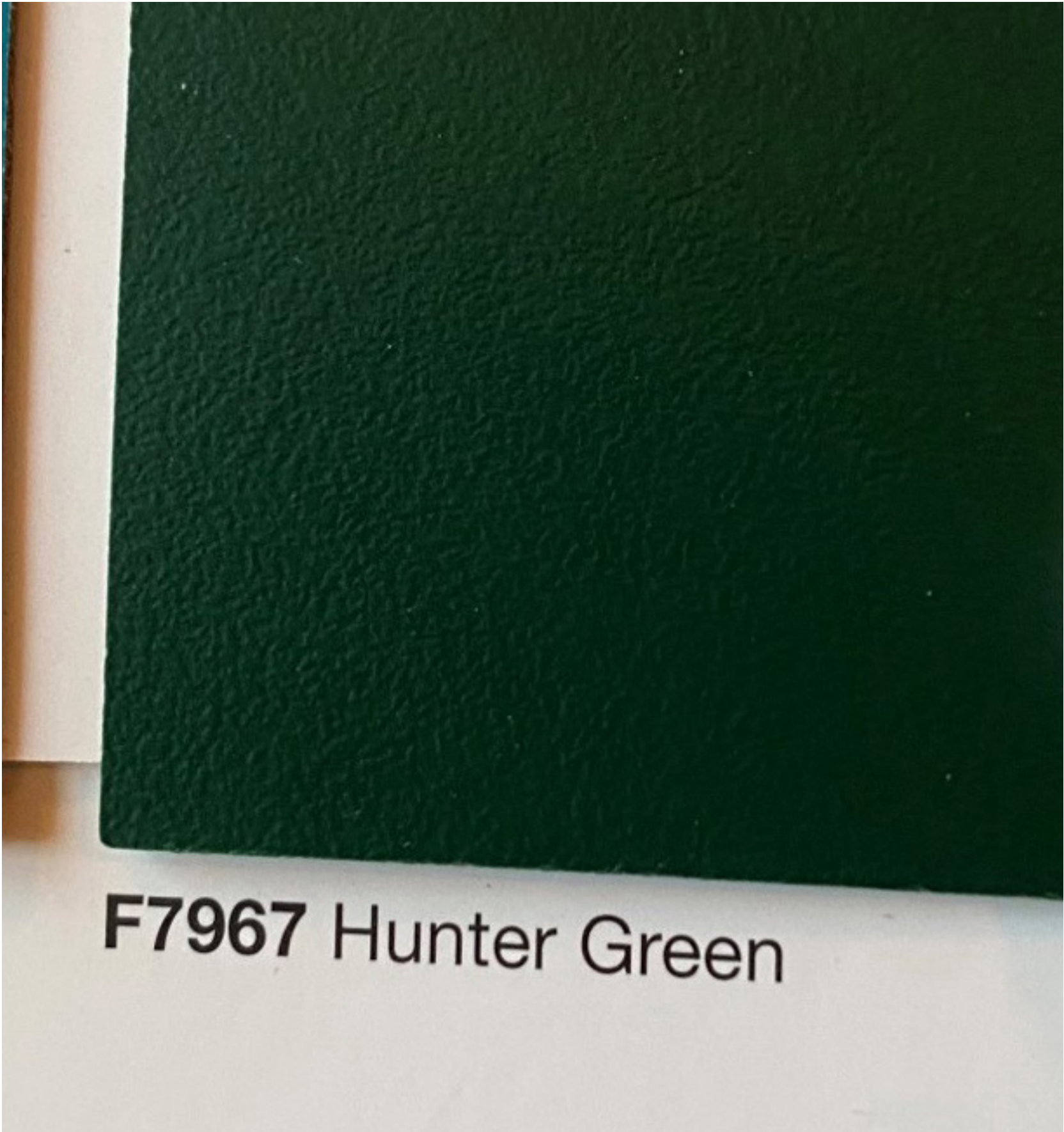
2.7 Back bar wall cladding: Dark Green (Hunter Green) Formica hygienic wall cladding This system is used for the back bar only, forming a neat panelised hygienic wall, creating a backdrop to the bar front and display shelving.
