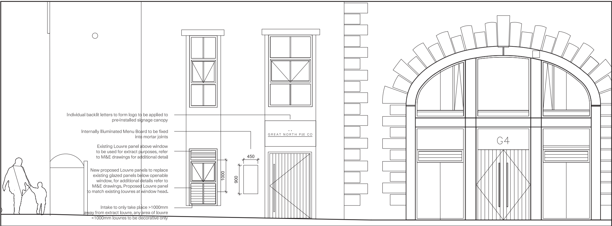
Proposed elevation to Little David Street (excerpt from drawing 13D showing elevation to Little David Street) - showing new louvre panels
