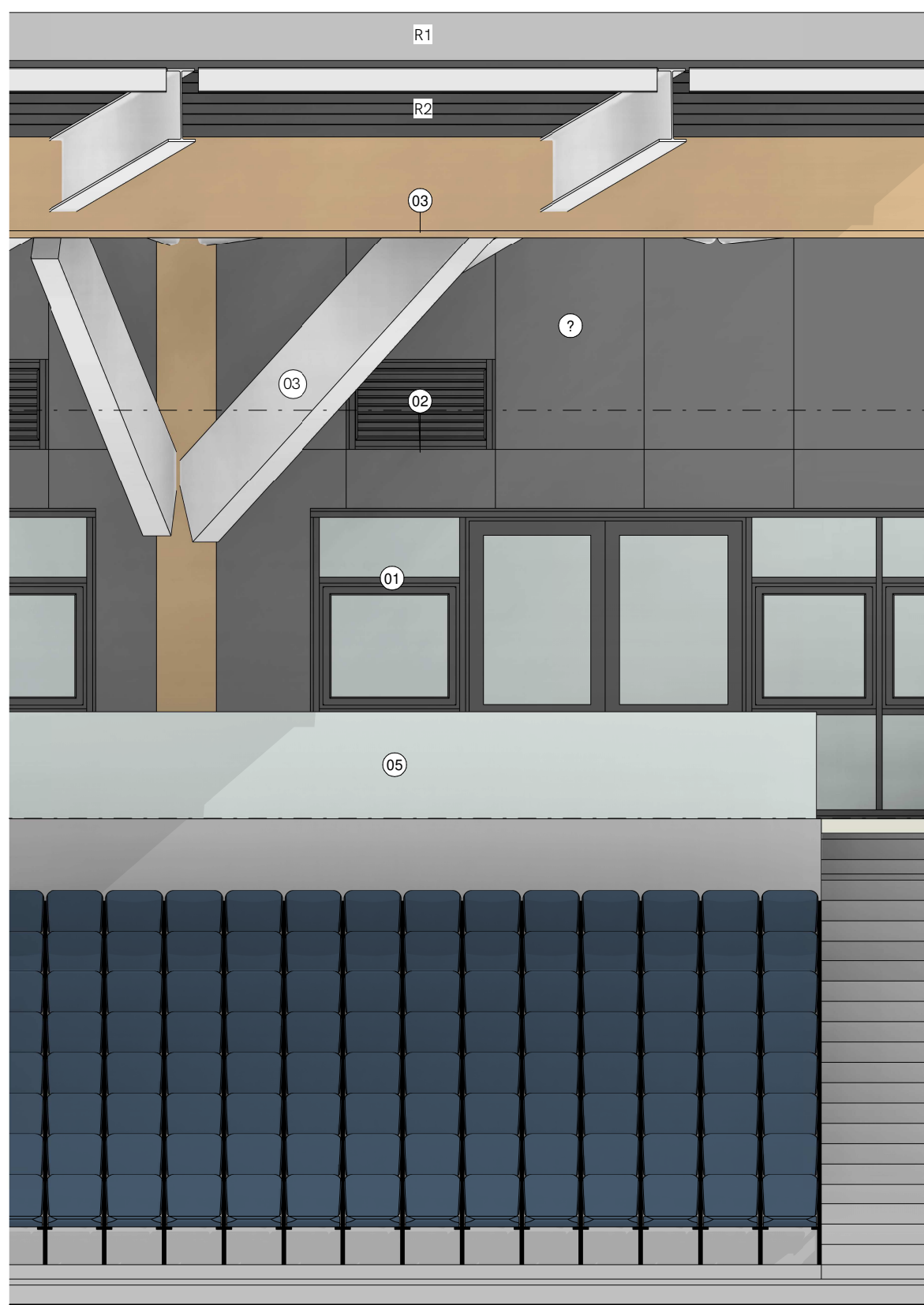
2 DETAIL WALL ELEVATION 1 1 : 50
