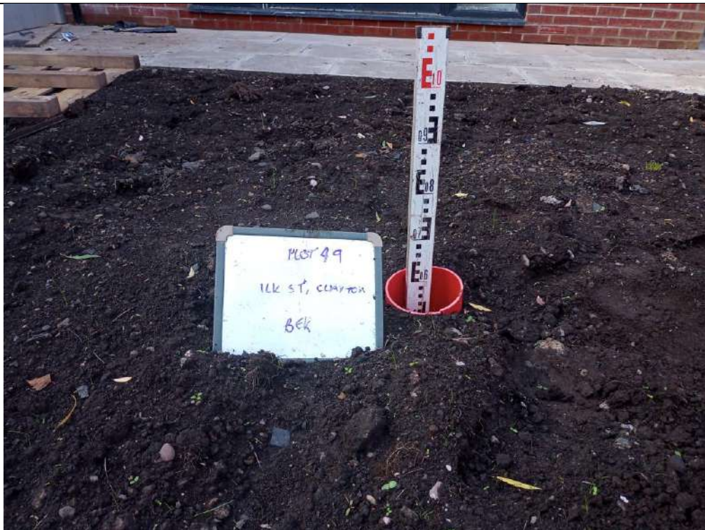
Photograph 1: Validation of Garden Capping Thickness
