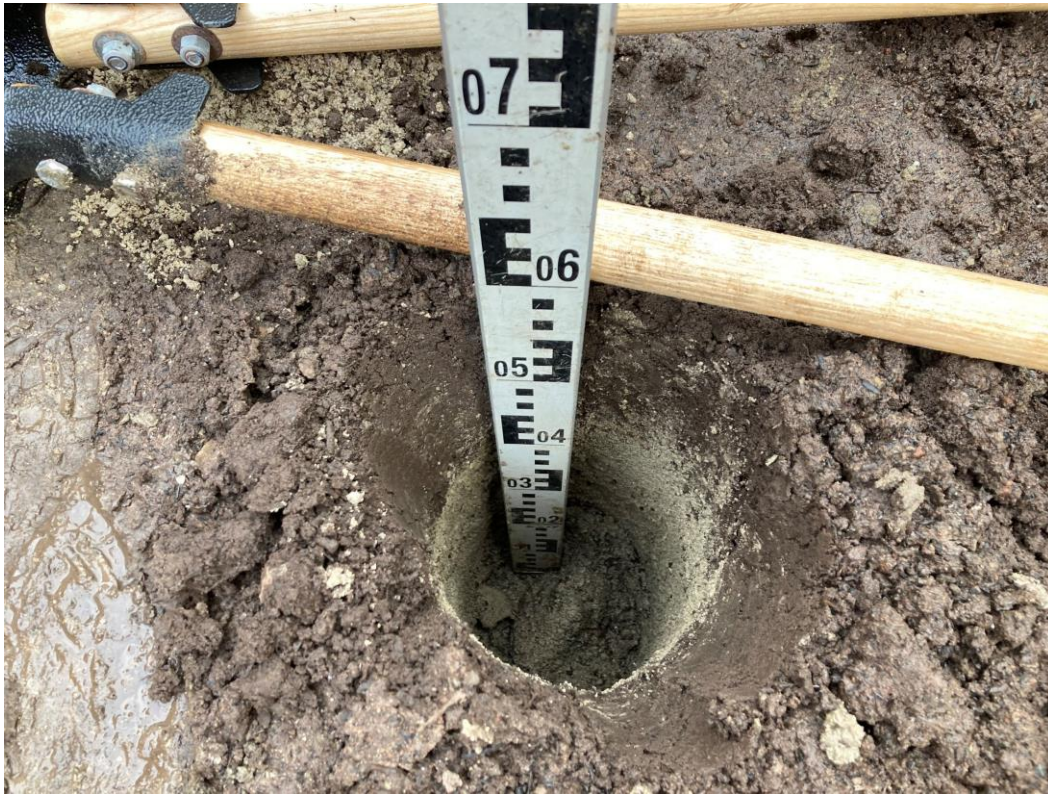
Photograph 5 VP03 showing 200mm of topsoil 400mm of subsoil.
