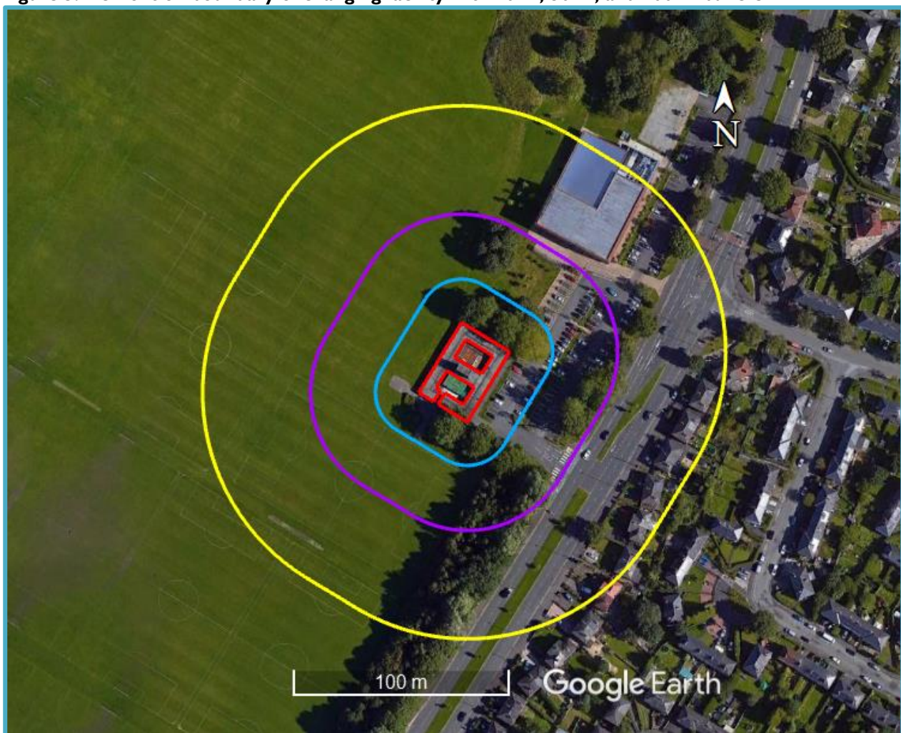
Figure 3. Demolition boundary of changing facility with 20 m, 50 m, and 100 m buffers
