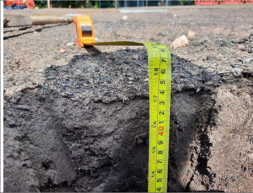
Plate 11: View showing depth of imported material at TS4/SS4.
