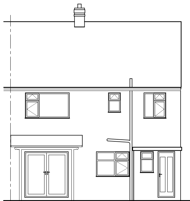
REAR ELEVATION AS EXISTING
