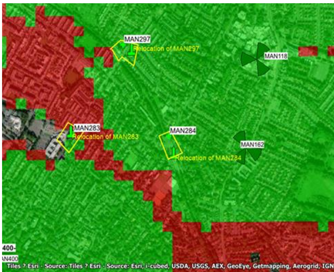
Figure 5: Cell Search Area Map with the Nominal illustrated by the green “T” marker labelled MAN284 below. The symbols labelled MAN118 and MAN162 are existing 3UK masts. The proposed equipment framed in this appeal can not be sited close to existing 3UK masts as the masts will interfere with each other. MAN297 and MAN283 are new site that are yet to be build. The proposed equipment also has to avoid these two locations as a new mast is to be deployed which will cause further interference if the apparatus is located to close to each other.
