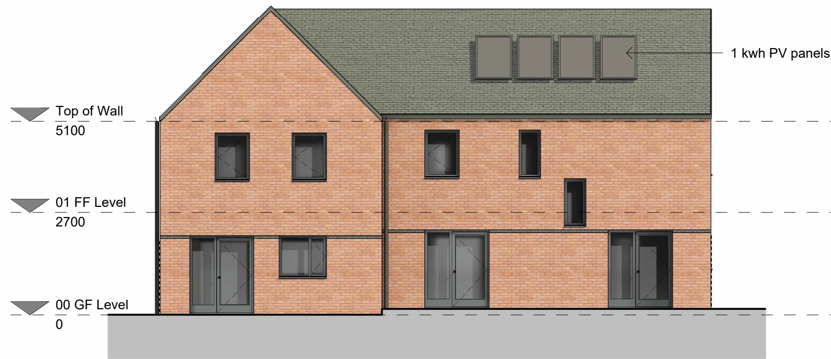
South Elevation / Rear 1 : 100
