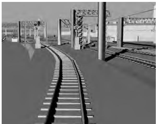
Fig. 06: Computer model of train tracks & signals from photogrammetry
