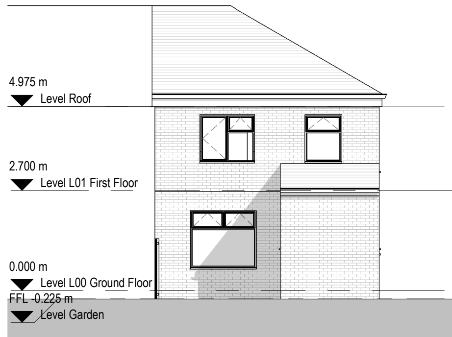
3 Existing East Elevation 1 : 100
