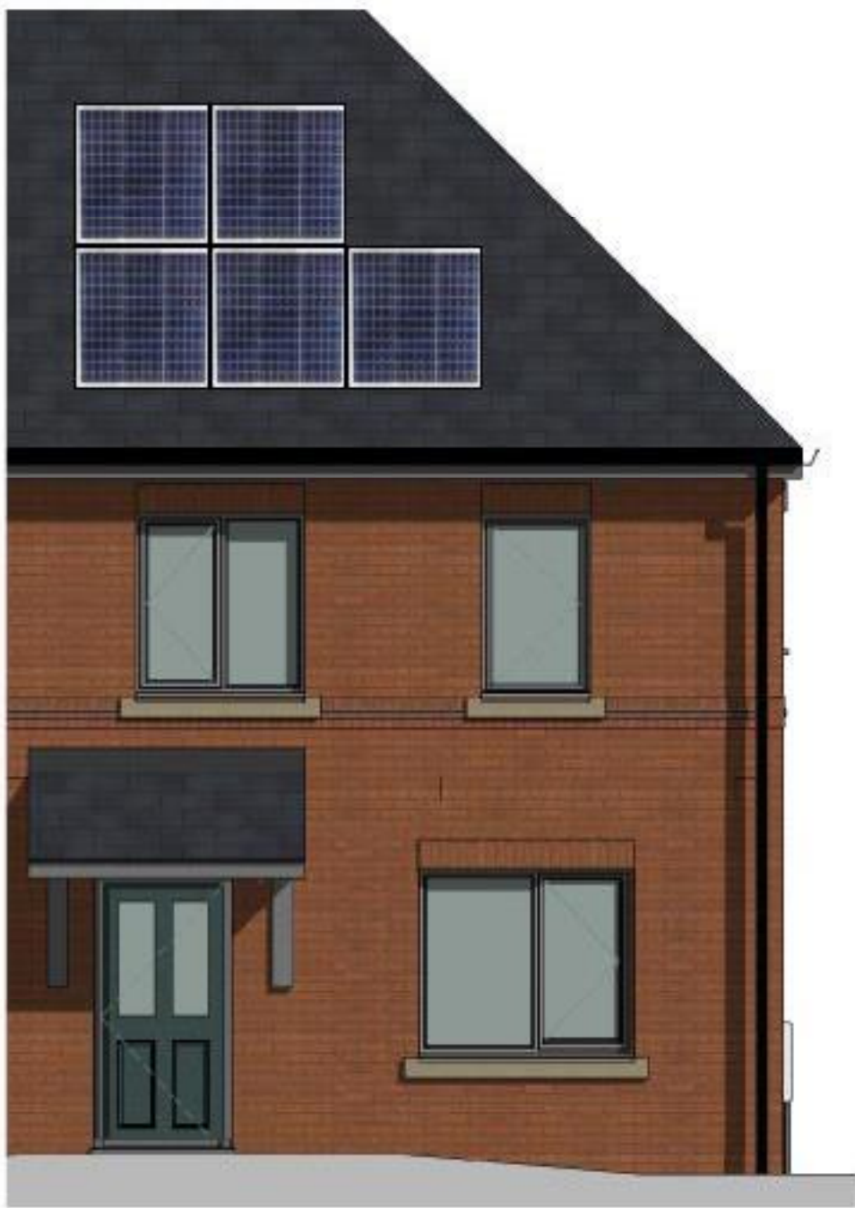
10 Front Elevation - Brick Type A Hipped Roof 1 : 50
