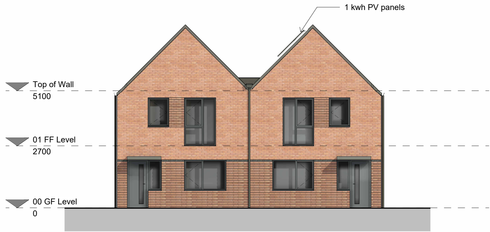
North Elevation / Front 1 : 100
