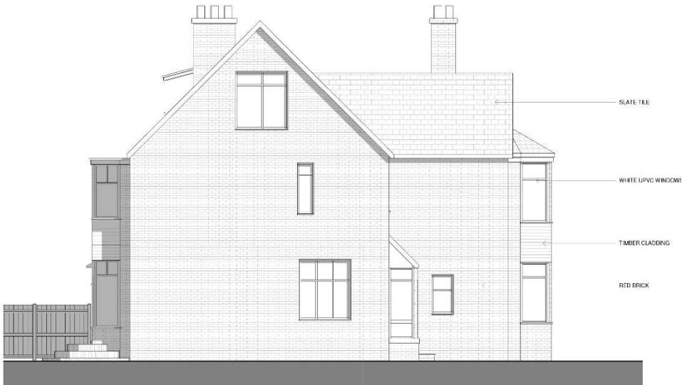
EXISTING ELEVATIONS - SOUTH-WEST 1 : 50
