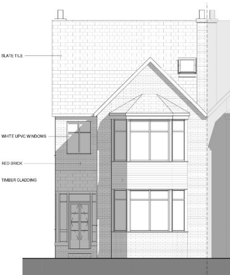
EXISTING ELEVATIONS - SOUTH-EAST 1 : 50
