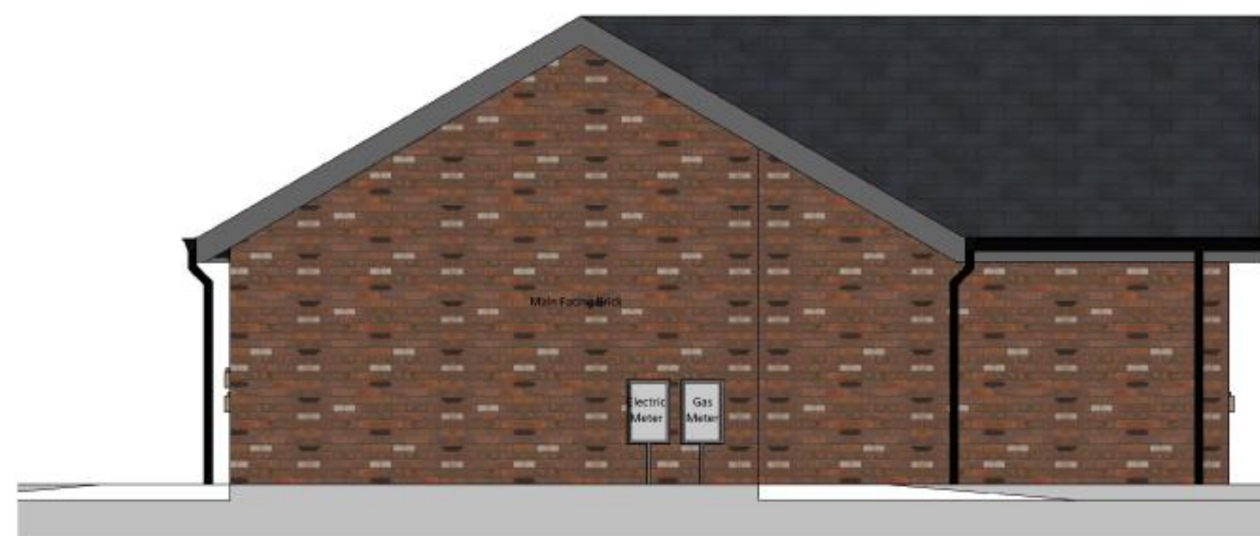
04 Gable Elevation 2 Brick Type B 1 : 50
