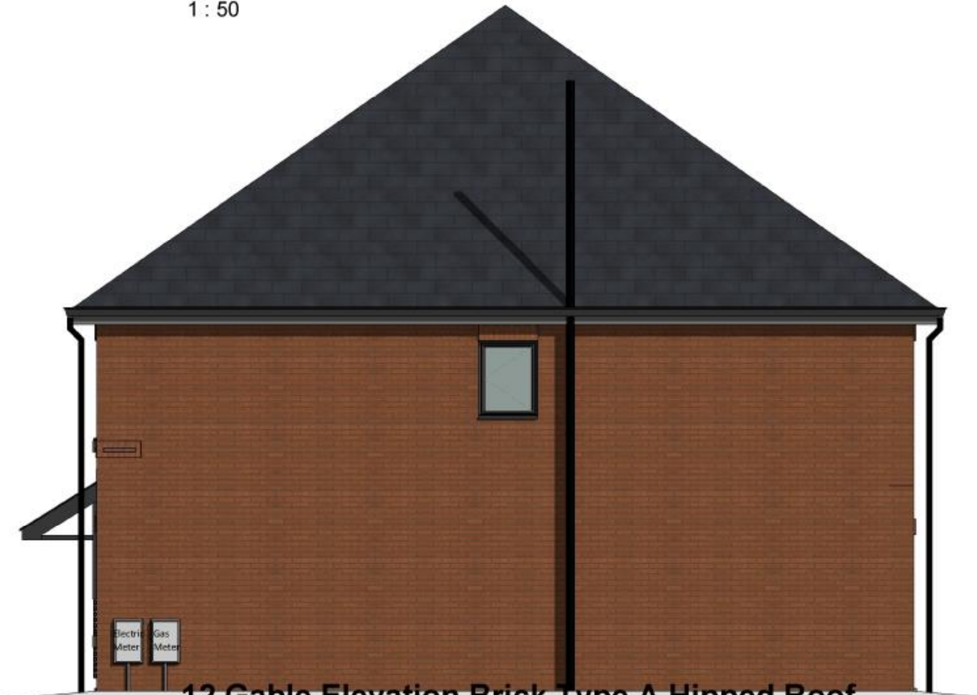
12 Gable Elevation Brick Type A Hipped Roof 1 : 50
