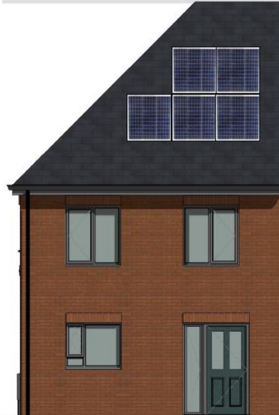
11 Rear Elevation Brick Type A Hipped Roof 1 : 50
