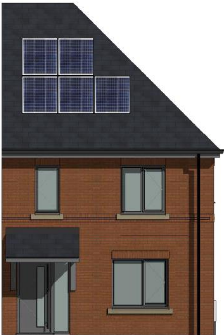
10 Front Elevation Brick Type A Hipped Roof 1 : 50
