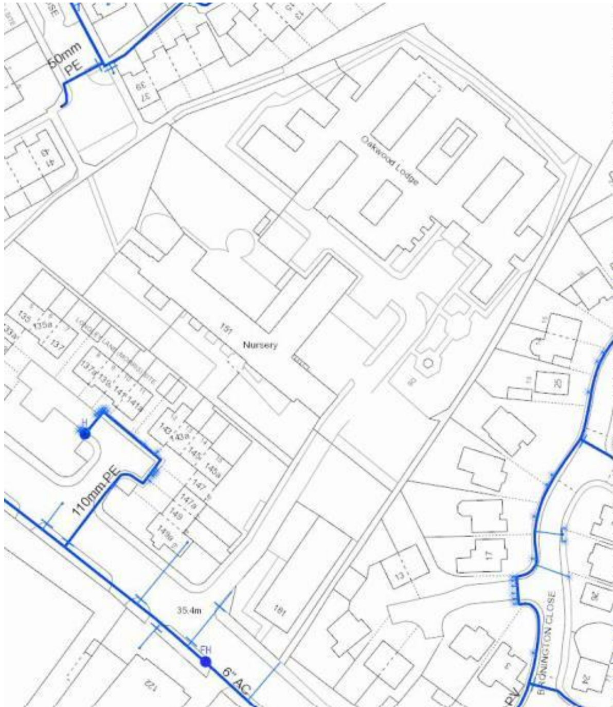
Figure 8.1 – Existing water infrastructure plan
