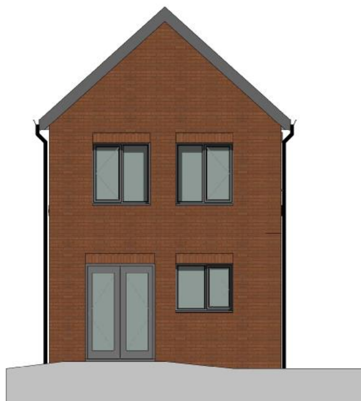
Rear Elevation Brick Type A 1 : 50
