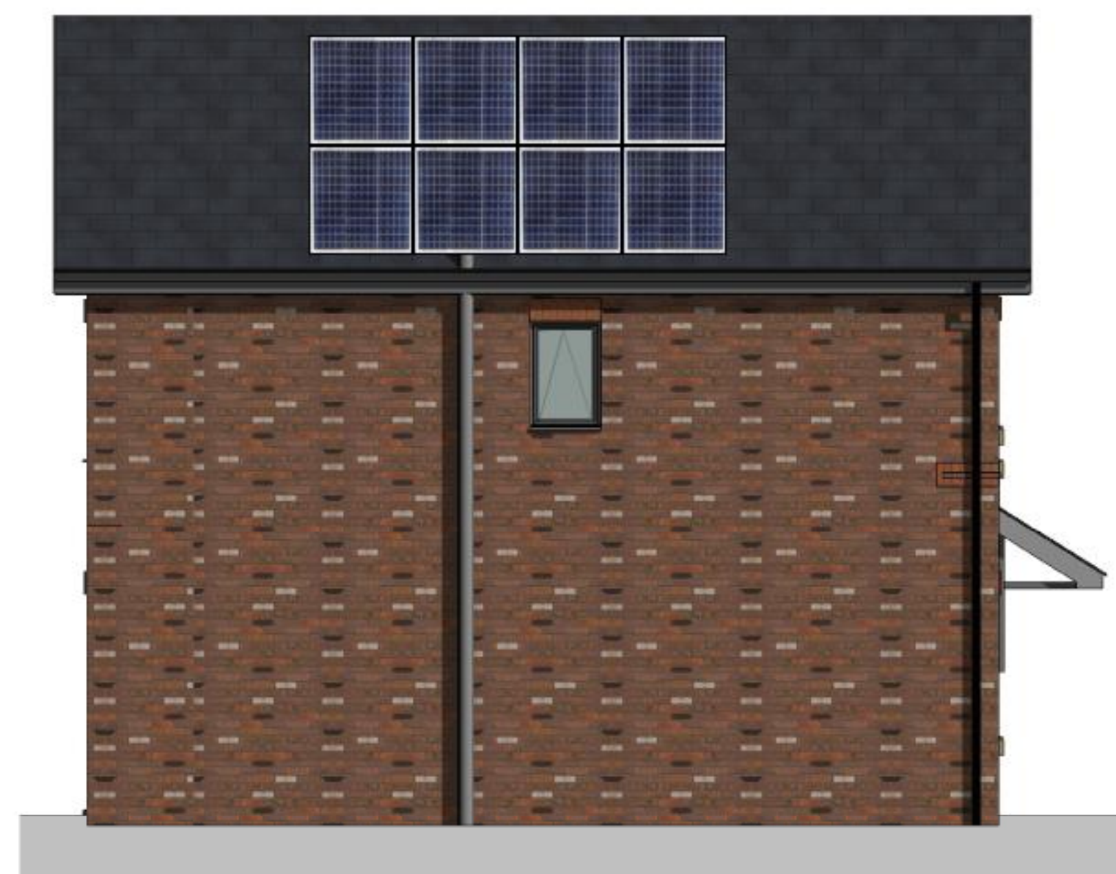
Gable Elevation - 2 Brick Type B 1 : 50
