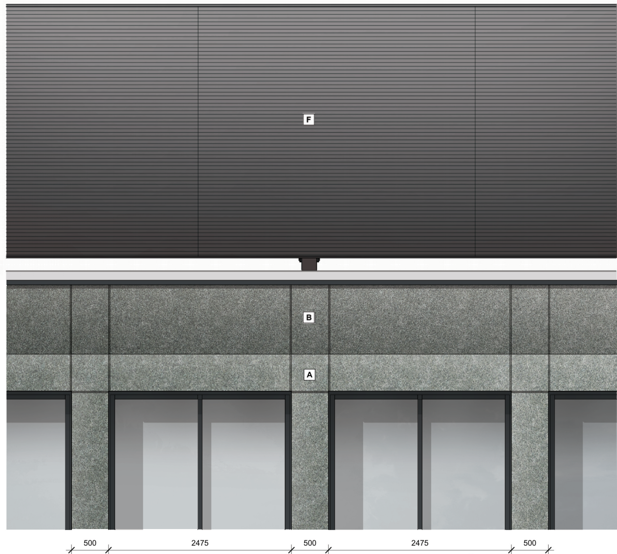
Parapet Plant Screen Elevation Detail 1 : 50
