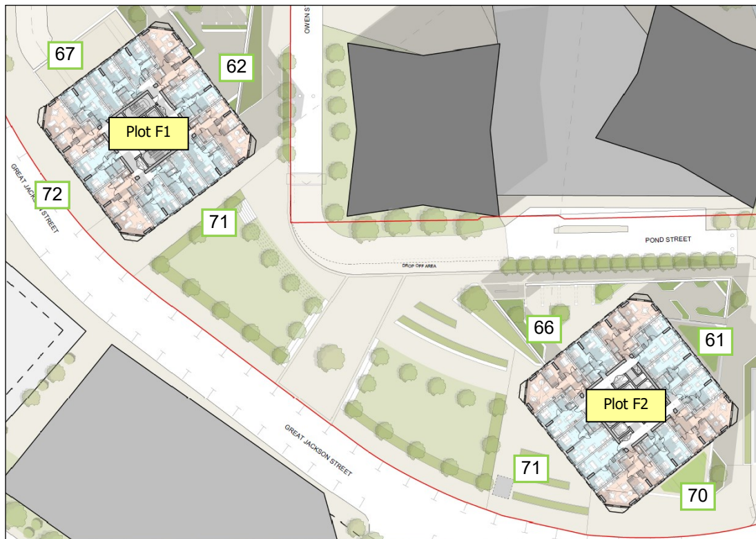
Figure 1: Summary external daytime noise levels incident on each façade (dB LAeq)
