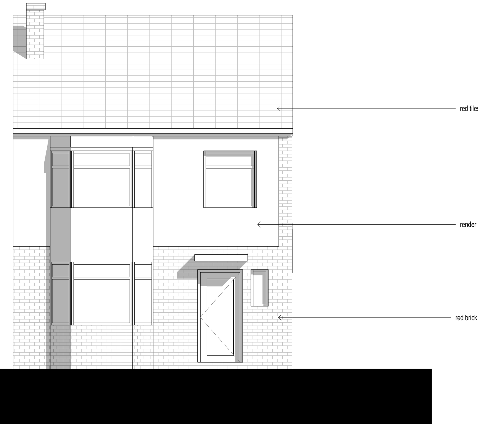
South Facing Elevation 1 : 50
