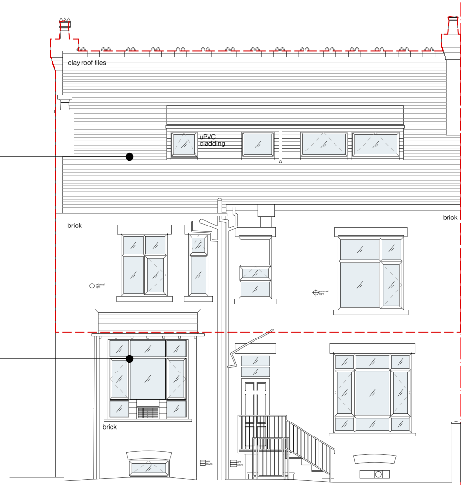
2 existing rear elevation 1:100 @ A3
