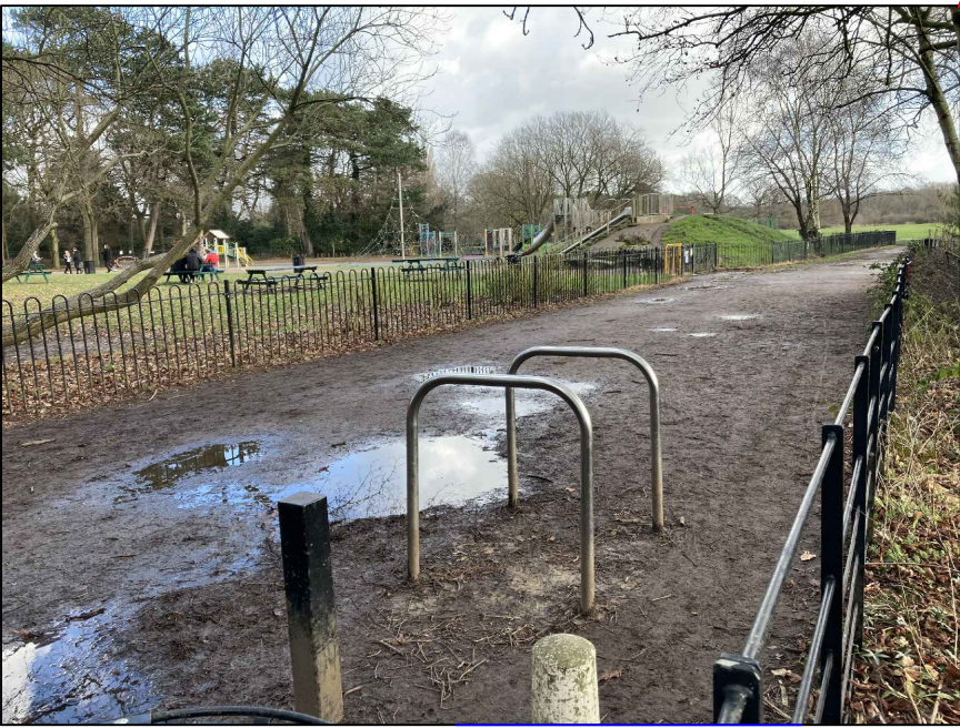
Photo 3: Existing cycle storage adjacent Children's Play Area comprising 2nr Sheffield stands; additional 3nr Sheffield stands to be provided. Total cycle storage provision of 5nr Sheffield stands.
