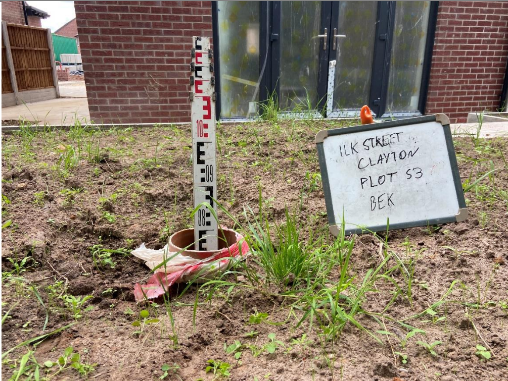
Photograph 1: Validation of Garden Capping Thickness (Plot 54, not 53)
