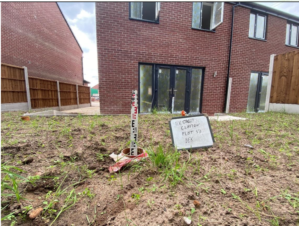
Photograph 2: Validation of Garden Capping Thickness (Plot 54, not 53)
