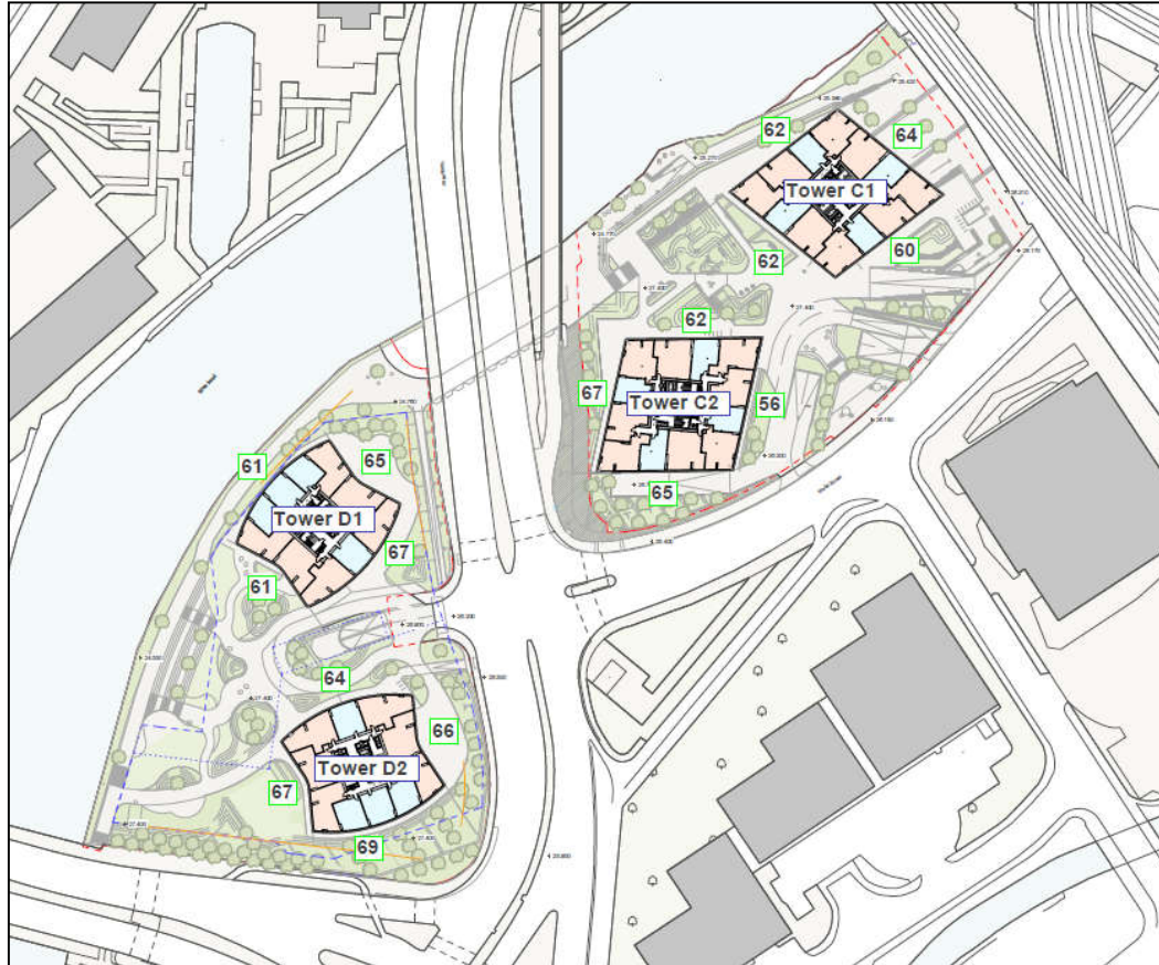
Figure 3: Summary external daytime noise levels incident on each façade (dB LAeq)
