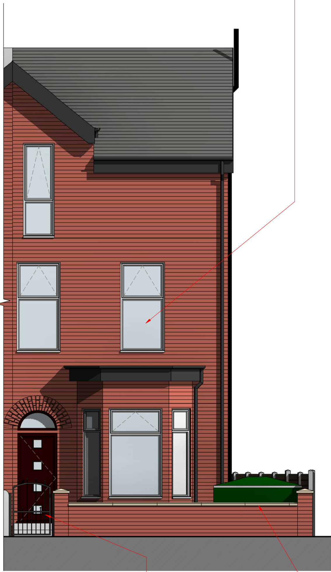
uPVC Double glazed windows. Colour: Anthracite Grey RAL 7016 with clear glazed or obscured panels.
