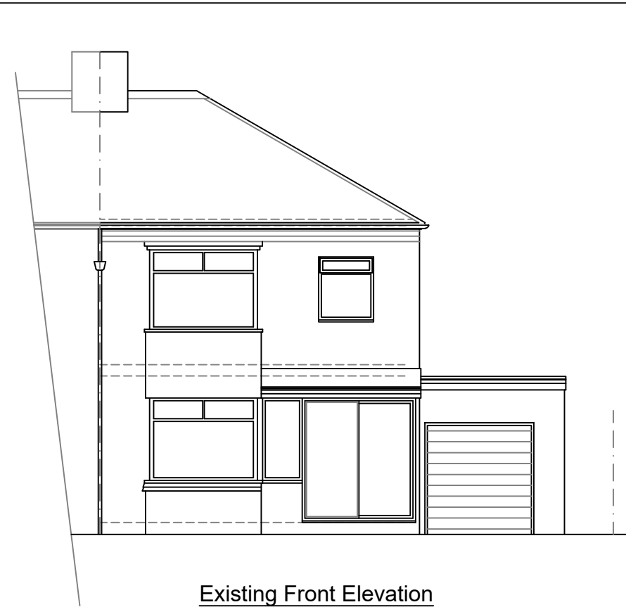
Existing Front Elevation
