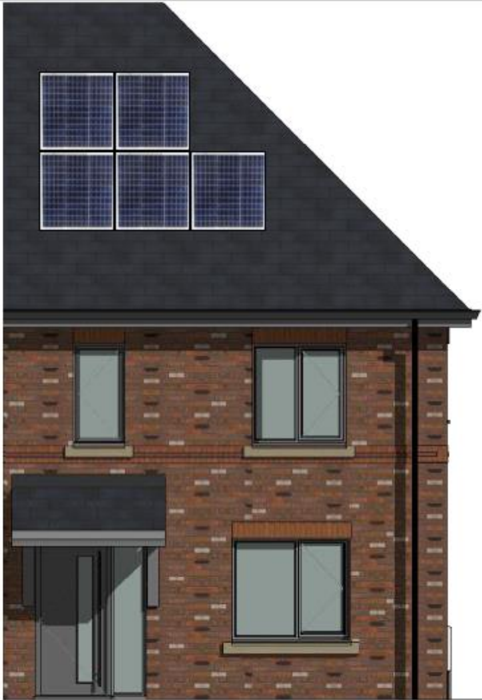
10 Front Elevation Brick Type B Hipped Roof 1 : 50
