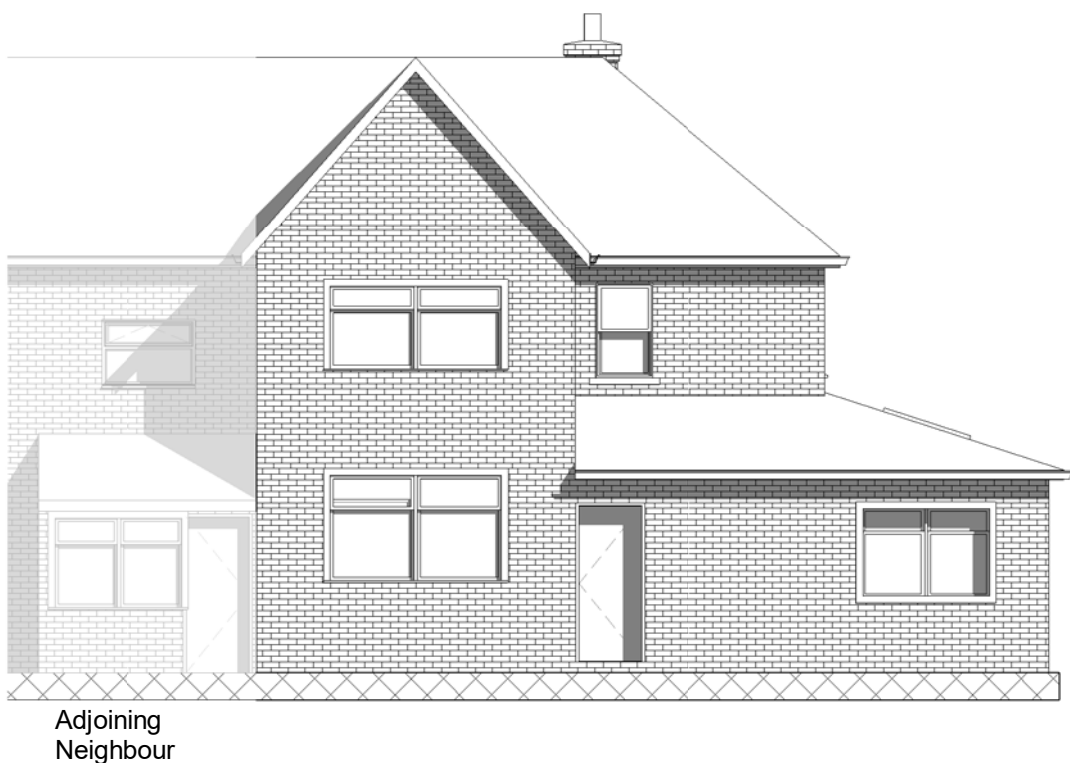
Existing Front Elevation 1 : 100
