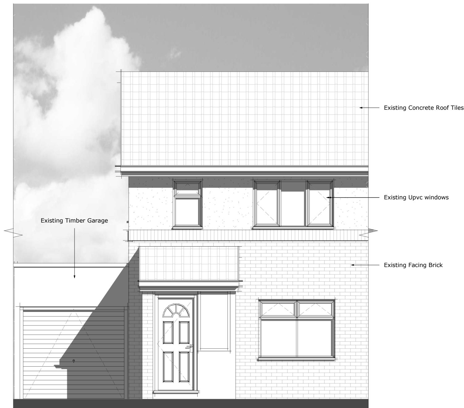
02 Existing Front Elevation
