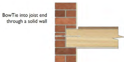
Image 2 - Helifix BowTie installation detail. Extract from brochure in appendix B
