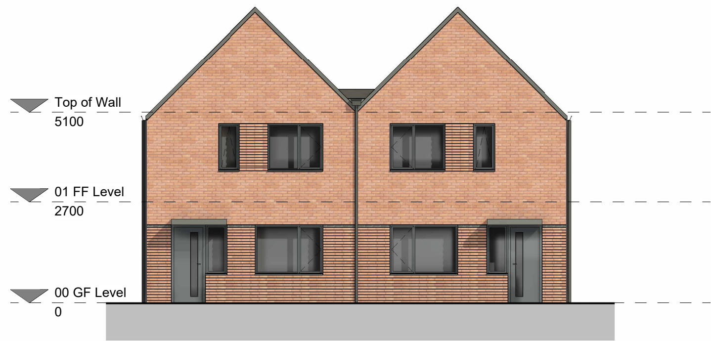
North Elevation / Front 1 : 100
