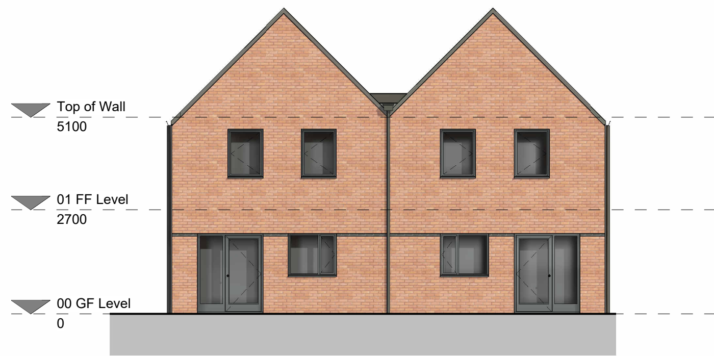
South Elevation / Rear 1 : 100
