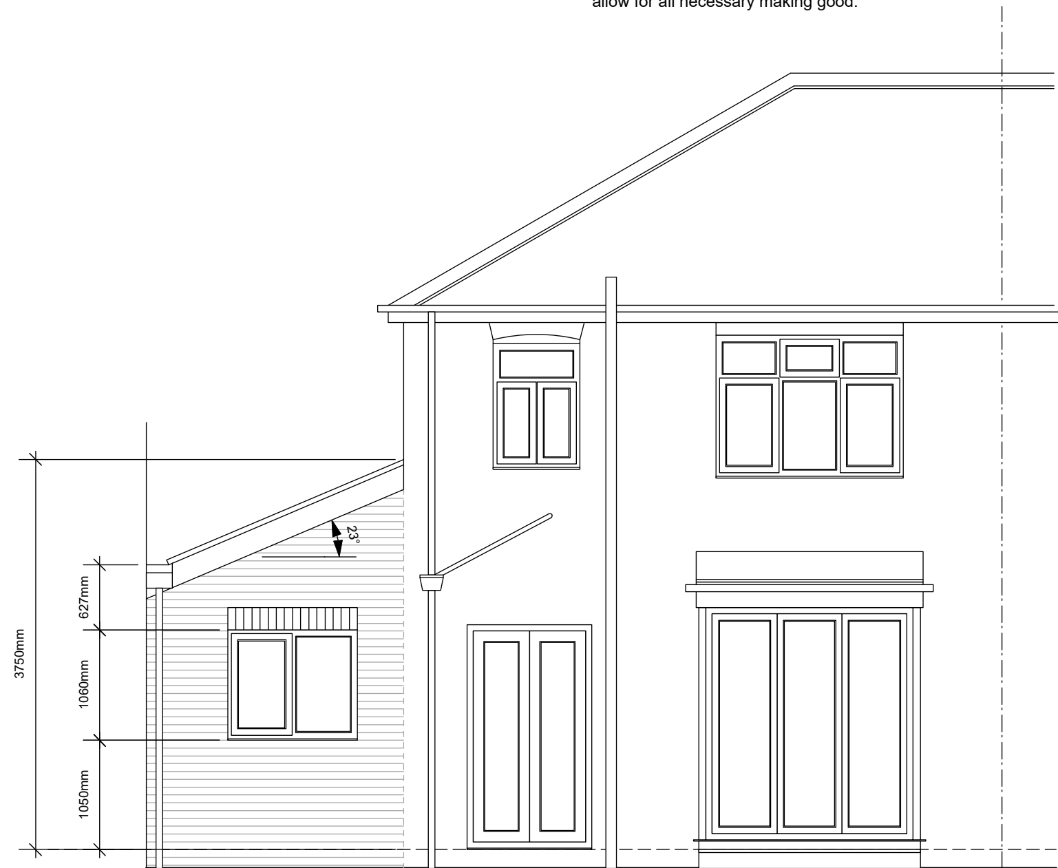
The existing kitchen window is to be carefully removed and external wall structure below the window sill, down to the ground floor level, carefully removed to form new french patio door set. The contractor is to allow for checkinng the existing lintel and repace if necessary. The contractor is to allow for closing the existing cavity at jambs with thermal cavity closers. The contractor is to allow for all necessary making good.
