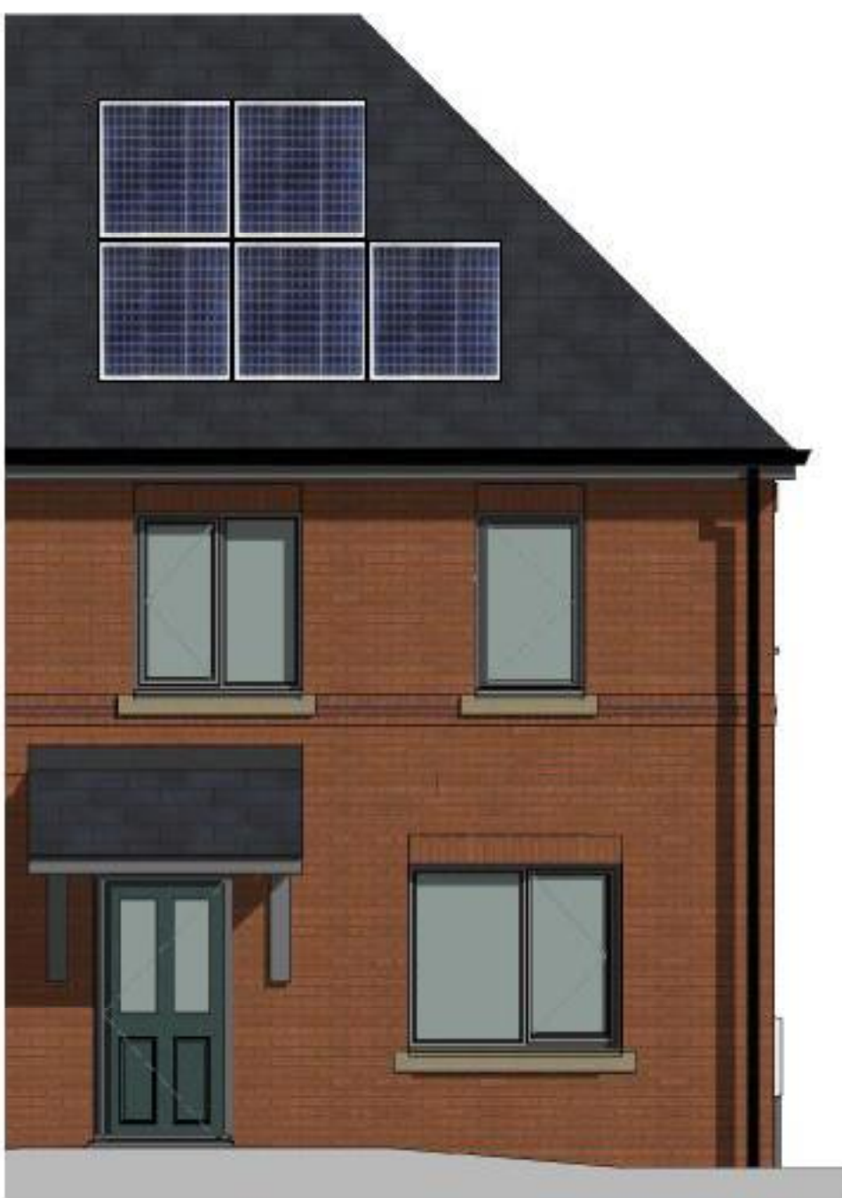
10 Front Elevation - Brick Type A Hipped Roof 1 : 50
