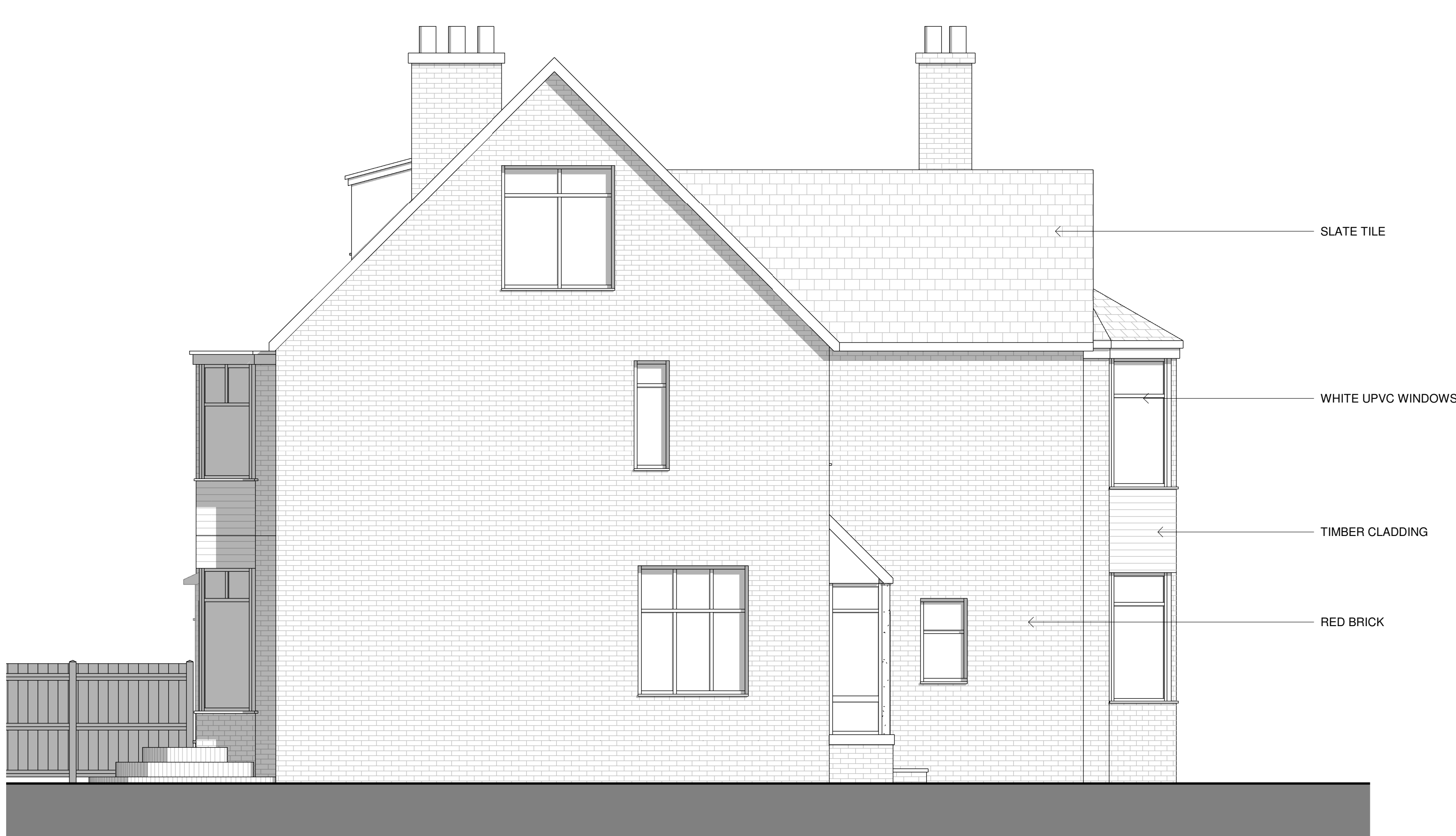
EXISTING ELEVATIONS - SOUTH-WEST 1 : 50
