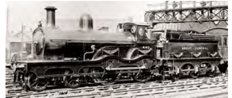
Charles Sacré's Class "6" 4-4-0 No. 440, built at Gorton Works in 1881 used by the MSLR
